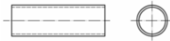
a) Full-section specimen
