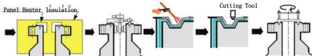
Local PWHT Machining of Gasket Groove WOL of Tp. 347L Finish machining of Final layer Finish by lapping of Gasket Groove, NDE (DT&PT)
